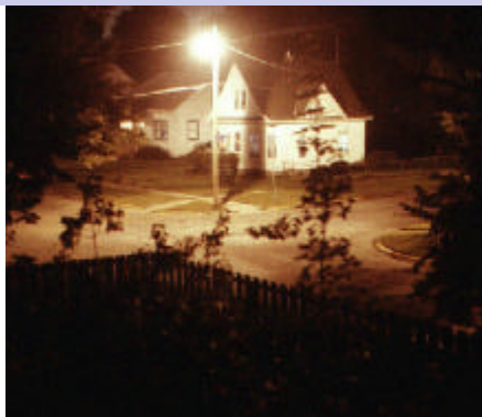
A streetlight before (left) and after installation of a full-cutoff fixture. The change is radical. Instead of seeing a dazzling bulb glaring sideways into your eye, you just see well-lit ground below — and sky above. Courtesy David Oesper (Outdoor Lighting Associates).
